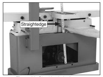
Figure 70. Checking belt alignment.
